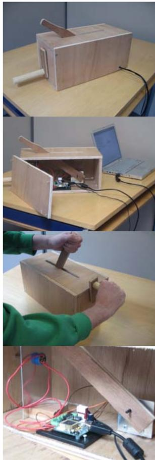
Fig. 8. The current prototype of the Croaker. From top to bottom: a view of the instrument, a view of the microcontroller and the sensors inside the instrument, use of the instrument and a close view of how the sensors are connected to the lever and crank.
