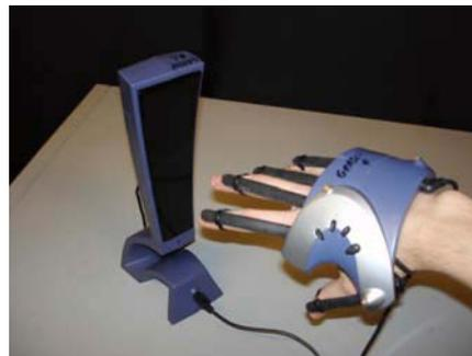
Fig. 1. The P5 glove controller
