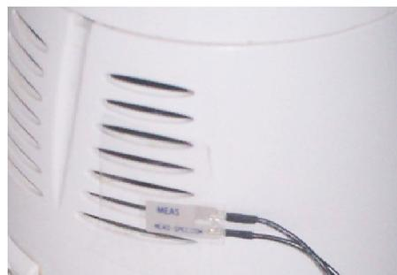
Figure 7. A piezo sensor attached to the rare engine grid of an electric blender.
