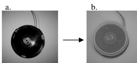
Figure 5. The temperature sensor (a) placed and (b) embedded in the plastic case for protection.
